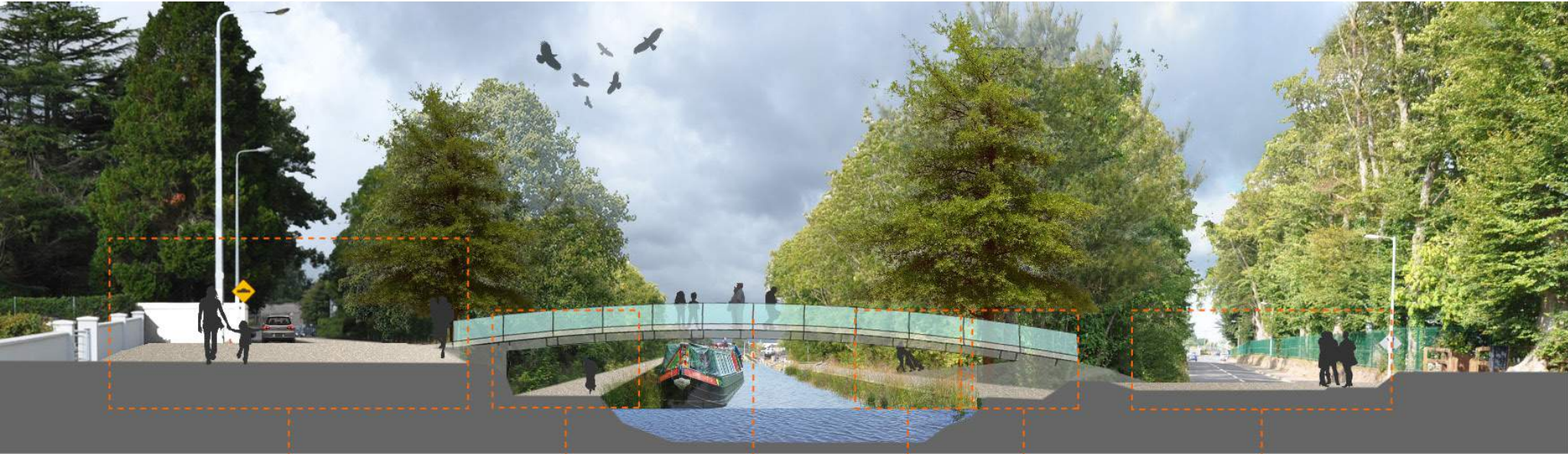
New raised table with continuous surface between school and bridge
